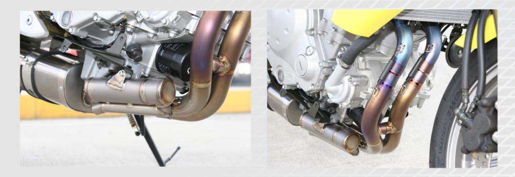
The Arata ER-6 full system features a titanium construction that incorporates a unique 'Remote Power Chamber' in its design. This helps increase peak horsepower on the ER-6 by reducing back pressure losses, inherant with the short mid pipe design of the stock system.
